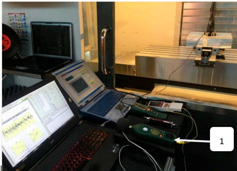
Figure 23. Test stand: 1 equipment for measuring of the sound intensity level.
