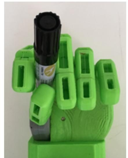
**Figure 14.** Centralized grip of the prosthesis while holding a pencil.
