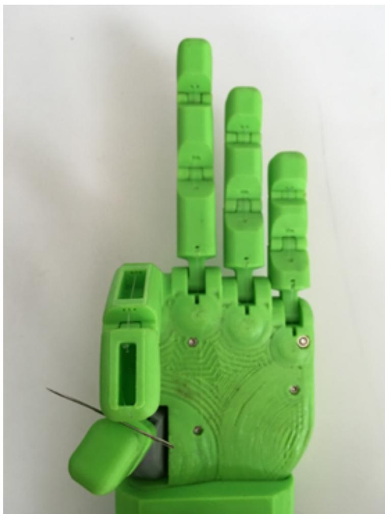
**Figure 9.** Prosthesis holding a needle through a bidigital opposition grip (terminal/terminal-thumbscrew dam).
