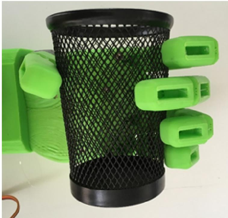
**Figure 13.** Full palmar grip while holding a conical object.
