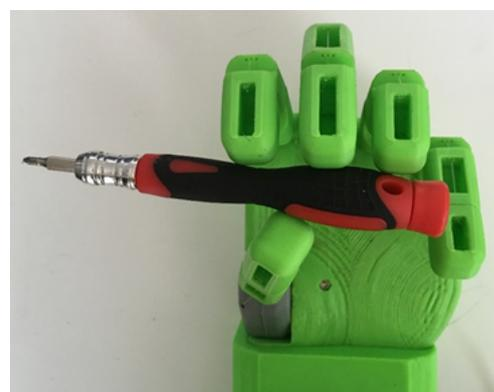
(b) Tetradigital thumb grip for holding a screwdriver.
