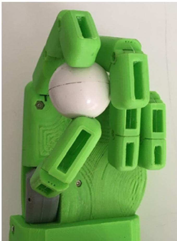
Figure 10. Prosthesis holding a sphere through a tridigital hold.
