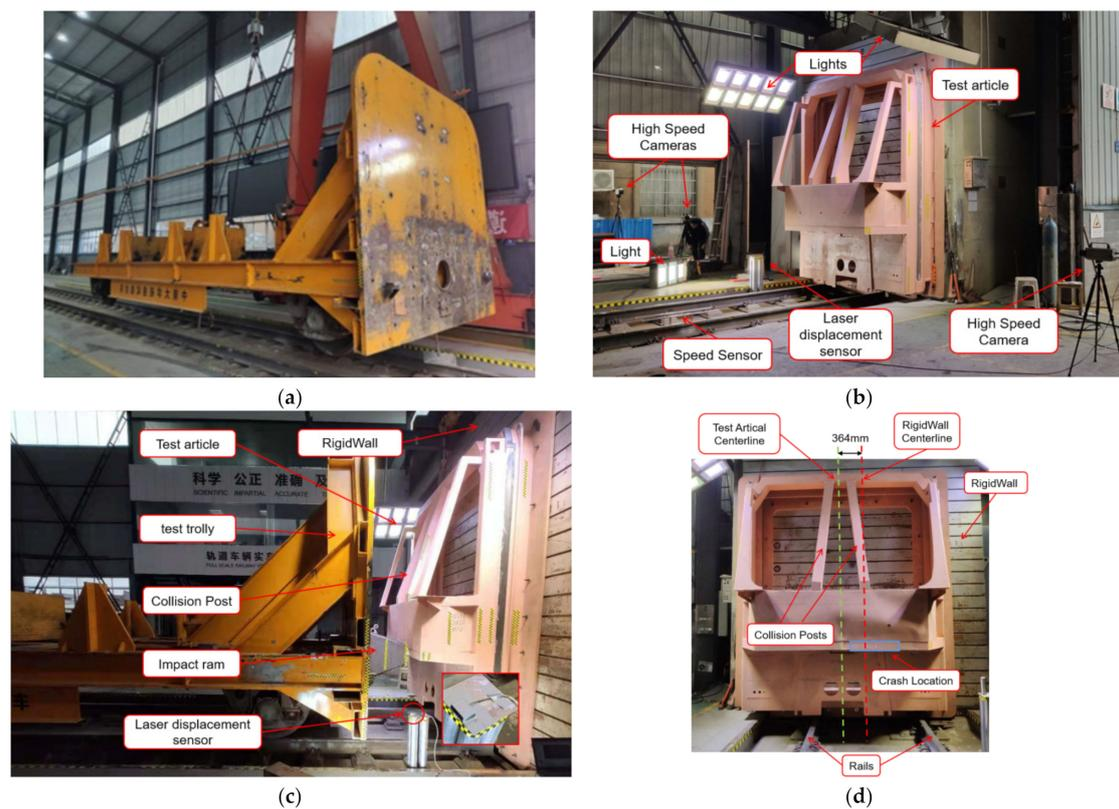
**Figure 4.** Experimental setup: (a) test trolley; (b) measurement devices; (c) crash location; (d) test article location.
