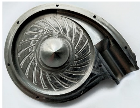
Figure 15. Processed blood pump casing with a hydrodynamic bearing.
