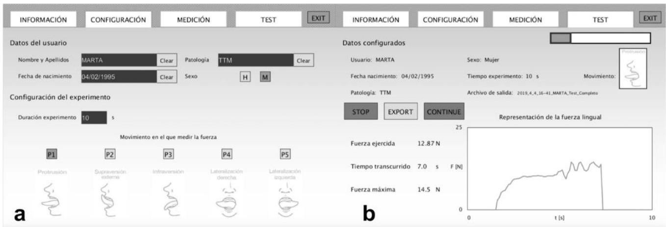
Figure 2. Spanish prototype device interface view. (a): Configuration screen view; (b): Measurement screen view.
