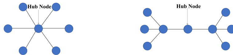
Figure 1. Illustration of a hub node based on the (left) degree and (right) betweenness centralities.
