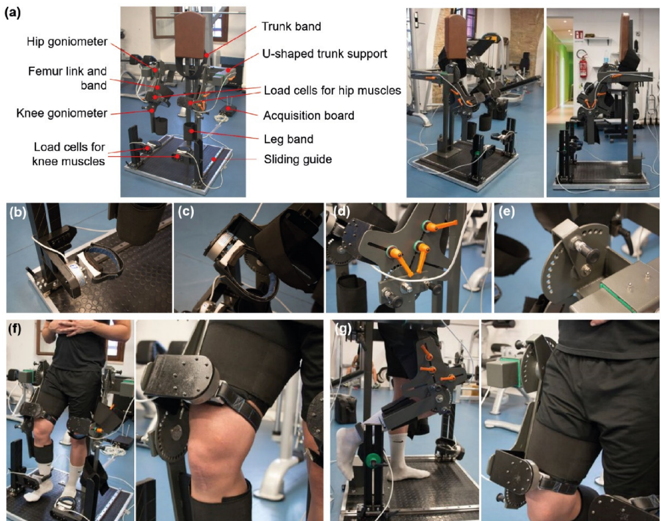
Figure 1. Description of the custom device to measure the isometric force used in this study. Scheme of the instrument with the critical components highlighted and pictures of the device from different viewpoints (a). Zoomed views highlight some essential components of the platform: load cell at the ankle (b); load cells at the knee (c); handles allowing one to adapt the machine dimensions to the subject anatomical characteristics (d); and goniometer to verify the flexion/extension degree of the joint (e). (f) Images of a subject undergoing a knee extensor force measurement test; (g) images of a subject undergoing a knee flexor force measurement test.
