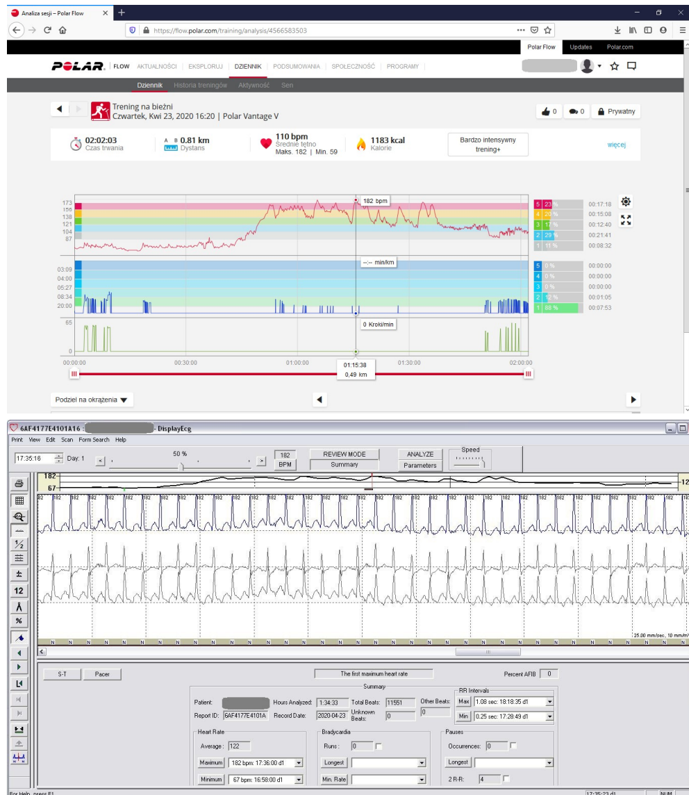
Figure 4. HRM control by comparing heart rate (HR) on HRM and at the same time in Holter ECG. The diagram with HRM indicates max. HR 182/min. At the same time, the Holter ECG indicates a rhythm of 182/min. The test was performed during a modified effort test on a treadmill. (number 8 in Table 4).
