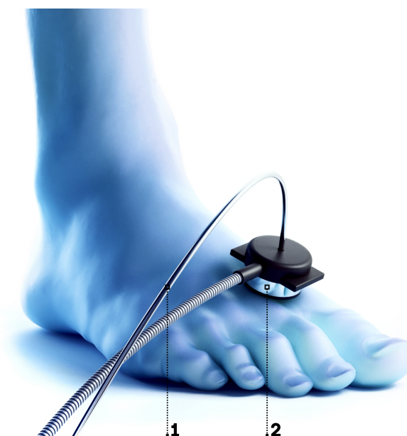
Figure 4. Allocation of the fibre optical probe combined with the attachment for the heat and cooling tests on the dorsal surface of foot. 1—fibre optical probe; 2—the attachment for the heating and cooling tests (contains Peltier element with water cooling).
