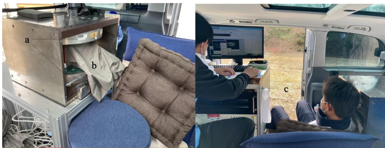
Figure 2. The mobile MRI system. (a) Permanent magnet. The magnet is a 0.2 T permanent magnet (NEOMAX Engineering, Japan; 200 kg; 16 cm-gap; 44 cm × 50 cm × 36 cm). The magnet was screwed onto an aluminum stand that was anchored to the sheet rail of the vehicle; (b) an RF probe was placed inside the conductive shielding cloths (ESD EMI Engineering Corporation, Tokyo, Japan). The home-built RF probe consisted of a solenoid RF coil (12 turns, 130 mm long, 94 mm in diameter) and a rectangular shield box (200 mm (x) × 200 mm (y) × 132 mm (z)) made of 200- \mu m-thick brass plates. The size of the RF coil was large enough to fit most of the junior baseball players; (c) MRI console: the MRI console consisted of a digital transceiver (DTRX6, MR Technology, Japan), a gradient driver (20 V, 10 A, DST Inc., Japan), a preamplifier (noise figure was 0.5 dB, gain was 30 dB; DST Inc., Asaka, Japan), an active transmit/receive switch, and a transmitter (9 MHz, 150 W; DST Inc.), which were installed on a 19-inch rack (56 cm × 77 cm × 60 cm, 80 kg). The MRI console was tightly fixed to the front seat with ropes.
