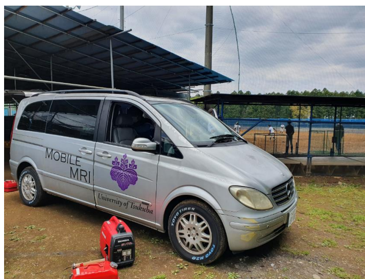
Figure 1. Photograph of the mobile magnetic resonance imaging (MRI) system beside a baseball field. (Mercedes Benz, GH-639811, width 191 cm, height 193 cm, and length 476 cm). Mobile MRI enables players to practice while awaiting their turn for an MRI scan.
