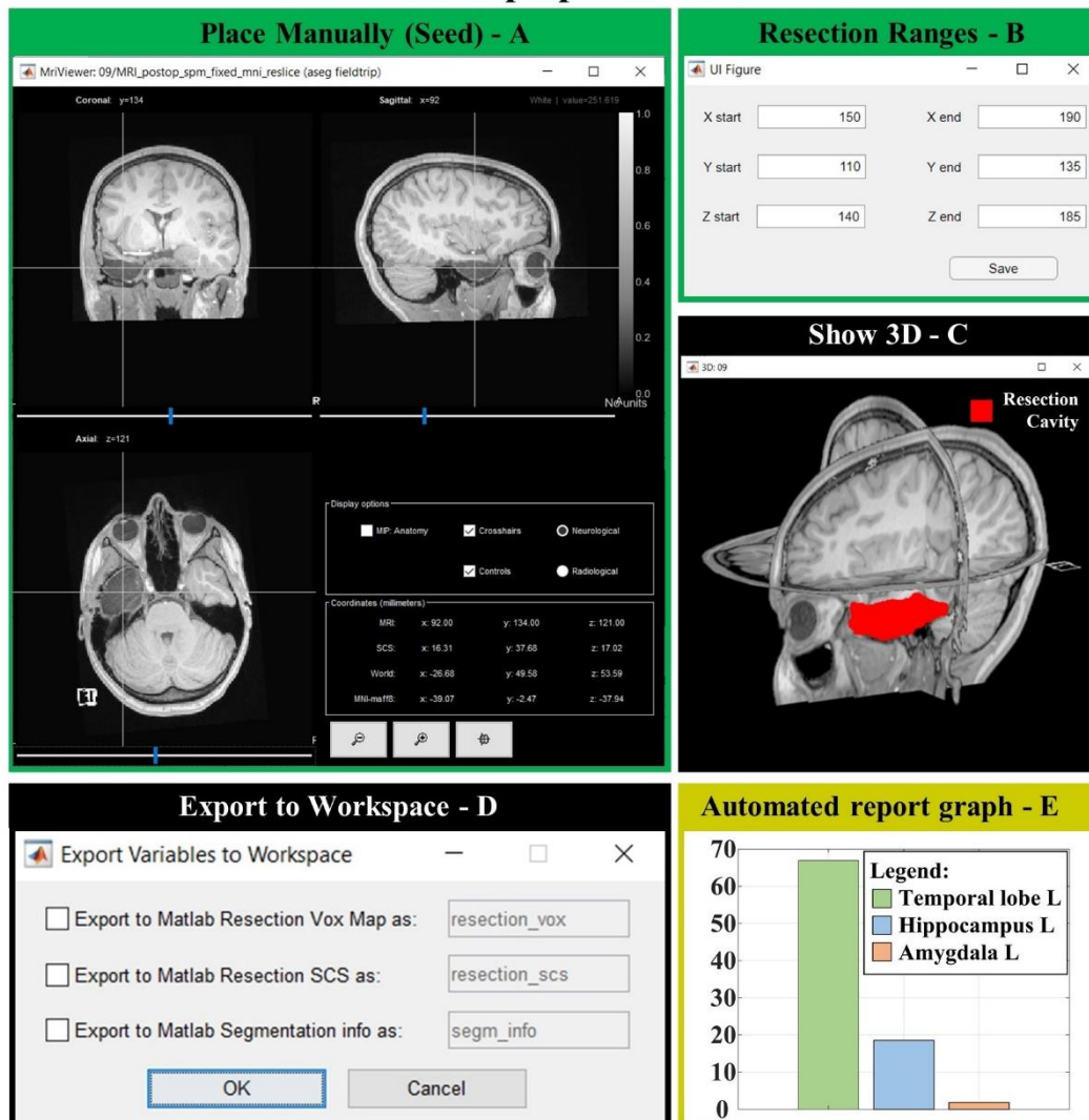
Figure 8. GUI popup windows. (A) MRI viewer for seed placement (when “Place Manually” is clicked). (B) Window for the definition of an optional ROI in which the region is free to grow (when “Change Ranges” button is clicked). (C) 3D MRI viewer from Brainstorm software (if “Show 3D” button is clicked) shows the 3D resection output (red). (D) If “Export to Workspace” is clicked, the user can export the output in voxel coordinates and/or in Subject Coordinates System (SCS), as well as the segmentation parameters and seed coordinates (Segmentation info). (E) Bar graph of the anatomical report (when “Generate automated report graphs” is selected).
