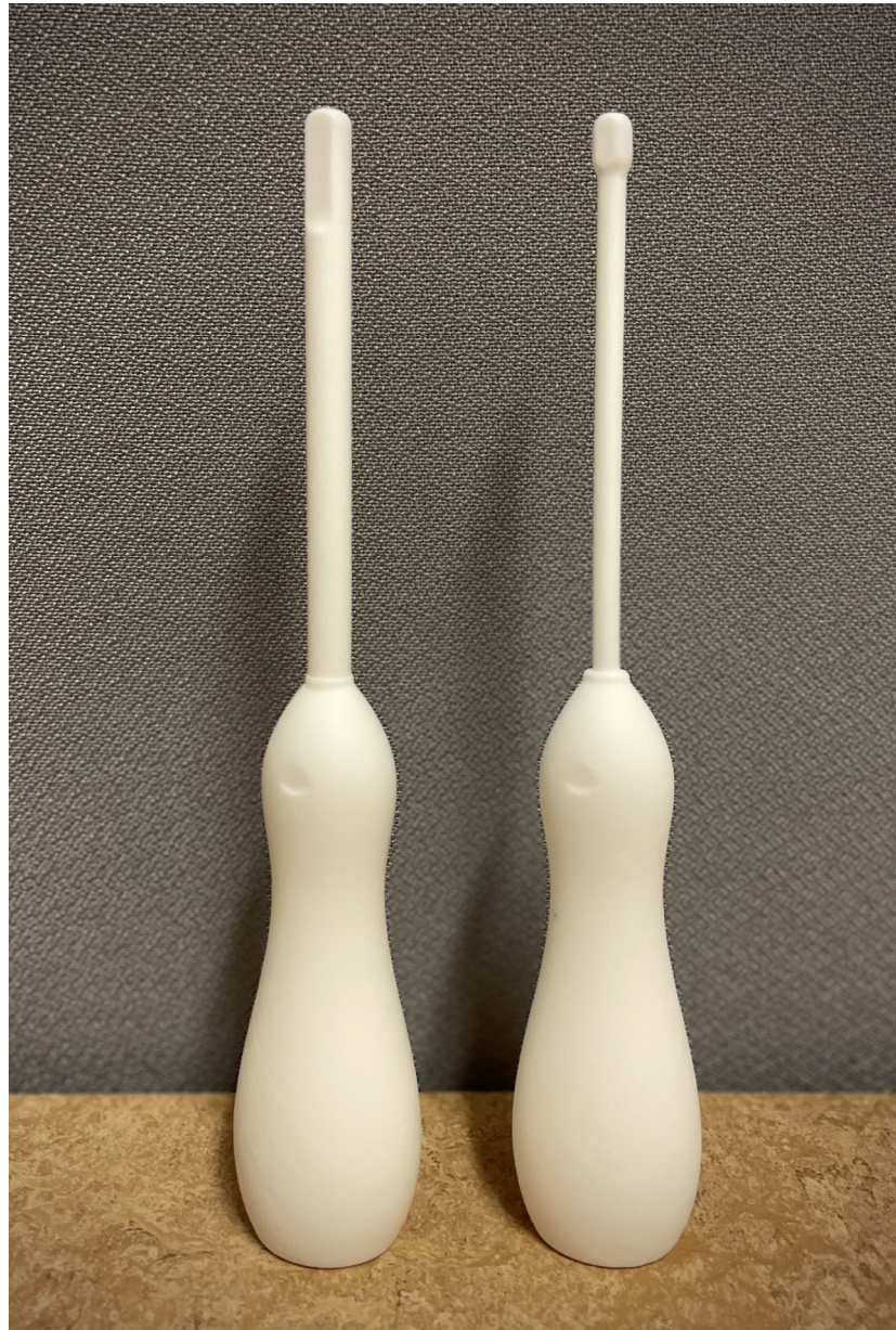
Figure 3. Two prototypes of a pediatric anorectal ultra-high frequency ultrasound probe. The prototype on the left has a head size of 8 mm and a shaft size of 8 mm. The prototype to the right has a head size of 7 mm and a shaft size of 5 mm.
