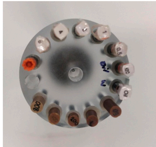
Figure 1. Photo of the calibration phantom. PMMA calibration phantom with eight 200 \mu L Eppendorf PCR inserts and five HA rod inserts.
