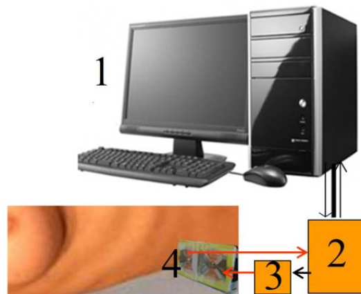
Figure 5. Measurements scheme: 1, computer; 2, oscilloscope; 3, generator; 4, receiving and transmitting antennas.
