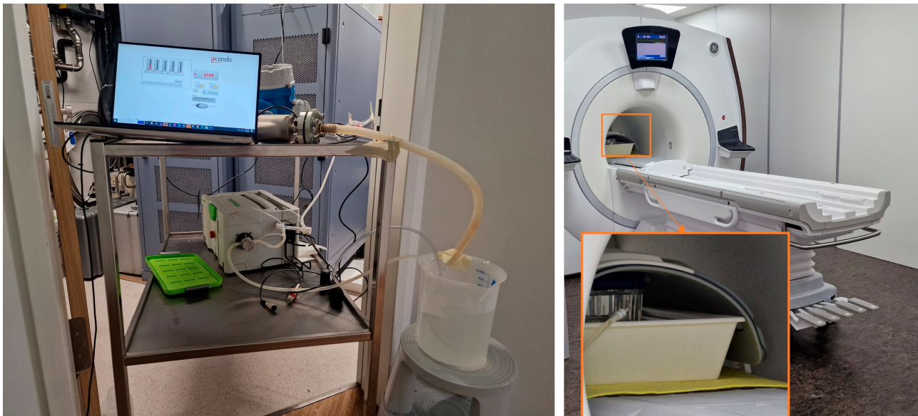
Figure 2. Flow phantom setup demonstrating the scanner (right) and the pump and the flowmeter in the control area (left).
