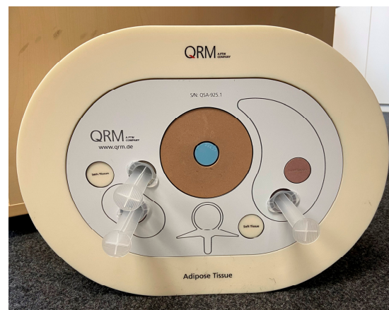
Figure 4. Test scan setup with obese extension ring. In the abdominal phantom, we fill three drill holes, each with one insert: One in the liver-equivalent region, one in the spleen-equivalent region, and one in the soft tissue-equivalent region. The inserts were cyclically swapped between the scans, mentioned in Table 1, to measure each one in all the different regions. The central hole of diameter 100 mm is filled by water-equivalent plastics.
