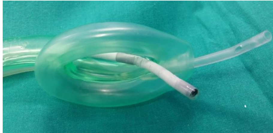
Figure 4. Distal end of the laryngeal mask airway. Exit of the fiberscope into the airway (white) and of the nasogastric tube into the esophagus (transparent).
