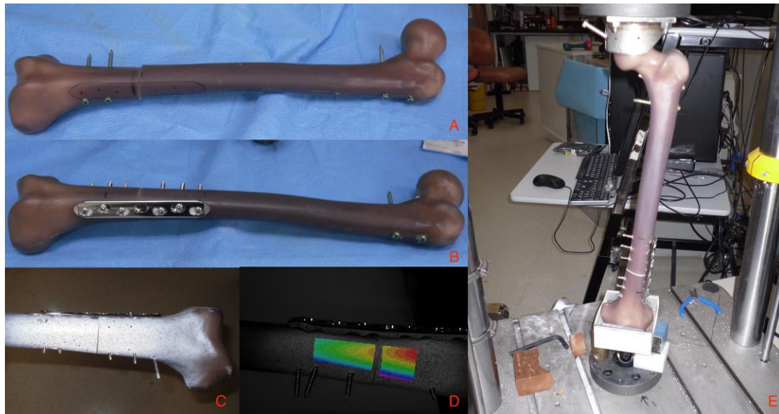
Figure 1. Test setting. (A) Preparation of the sawbone femora, with the nail in situ and an artificial fracture applied. (B) An additional plate is mounted. (C) The anterior surface of the bone is sprayed with a speckle pattern. (D) The system allows full-field 3D-surface strain and motion detection down to 200 \mu strain. (E) Sawbone femora are potted in PMMA distally and held by a universal joint that constrained translation and axial torsion but allow rotation in the other two axes. The femoral head is held in a custom fixture rigidly attached to the load cell. The axis of the bone is aligned in 7° valgus to the rotational axis of the testing machine to recreate a loading situation as close to physiology as possible.
