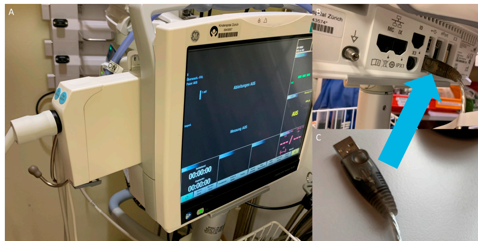
Figure A4. EEG module in side port of GE Carescape B450 (A), USB connection ports (blue arrow) at the rear of the GE Carescape B450 for data recording (B); USB cable for data recording, (USB to RS-232 Adapter, UC232A, ATEN, Taiwan; (C)).
