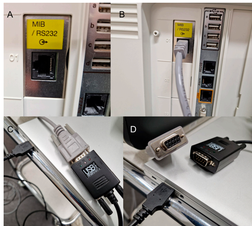
Figure A1. Data storage Philips IntelliVue system MX700. (A) Data port MIB; (B) Dataport with network cable (RJ45 to serial); (C,D) RJ45 to RS232 (grey, female) connector and USB to RS232 connector (black, male).
