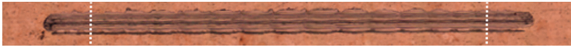
Figure 3. Wear track on OFHC copper disk showing the 4 mm length used for wear volume calculation.
