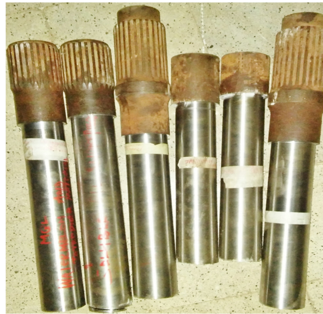
Figure 6. Machined AISI 1525 steel.
