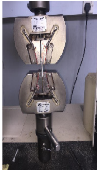
Figure 3. Tensile testing of AISI 1525 steel.
