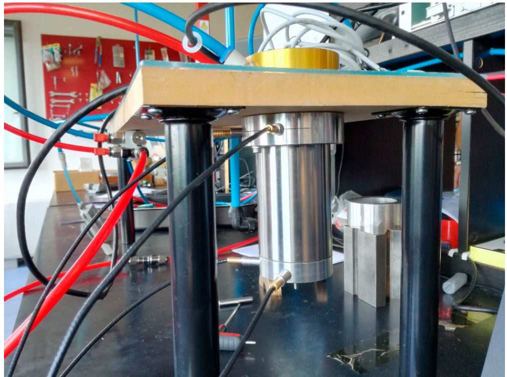
Figure 1. The electro-spindle under test.
