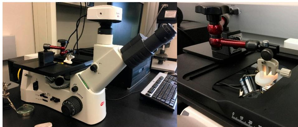
**Figure 3.** Stereomicroscopy Using a Universal Arm to Hold the Liners.
