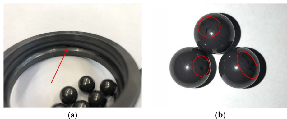
Figure 12. Outer ring raceway and rolling bodies of full ceramic ball bearing after the test. (a) Bearing outer ring raceway, (b) Rolling bodies.
