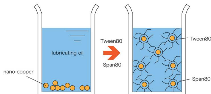
**Figure 7.** Modification process of nano-copper particles. Reprinted with permission from Ref. [34], Springer Nature.
