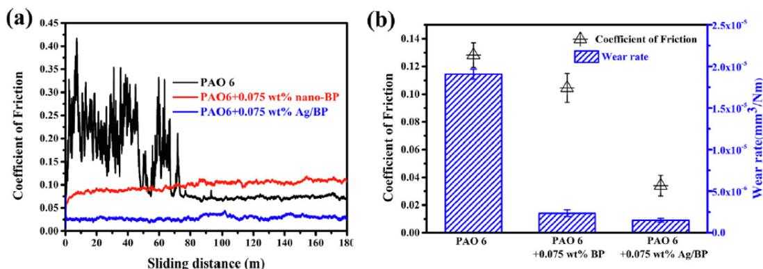
**Figure 8.** (a) Coefficients of friction versus sliding distance; (b) Average coefficients of friction and wear rates for the pure oil and oil samples with different nanoadditives (0.075 wt.%). Reprinted with permission from Ref. [50], Elsevier.
