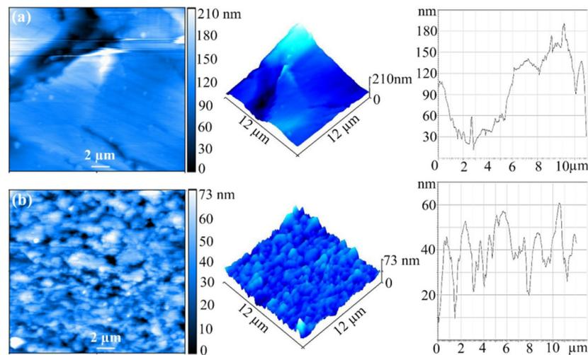
**Figure 4.** AFM results: (a) Original surface; (b) Surface after friction. Reprinted with permission from Ref. [15], Springer Nature.
