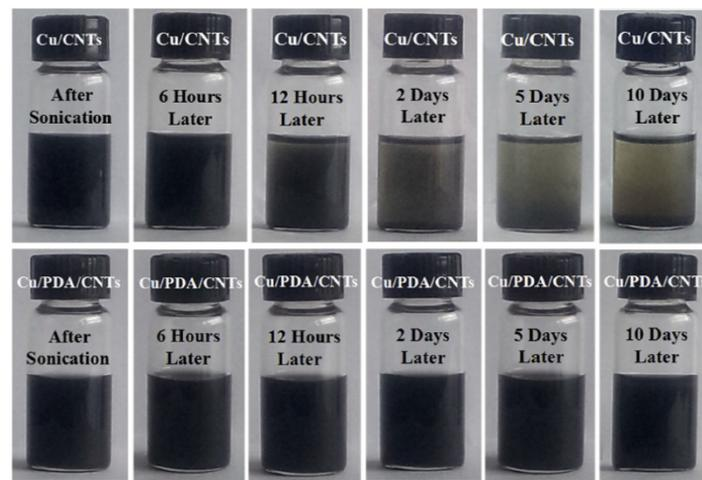
**Figure 11.** Dispersion performance of 0.2 wt.% Cu/CNTs and 0.2 wt.% Cu/PDA/CNTs in the base oil. Reprinted with permission from Ref. [56], Elsevier.
