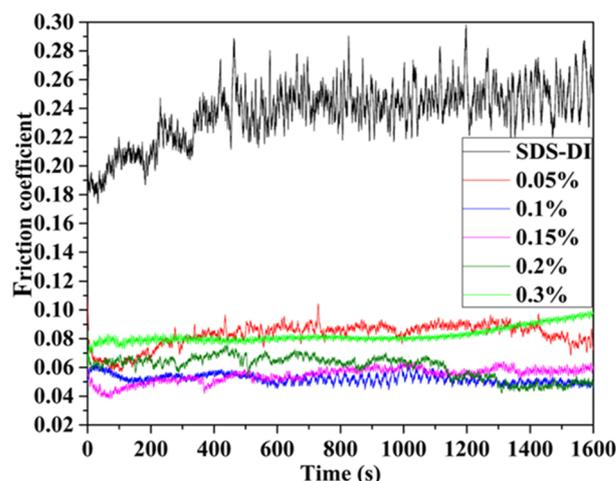
**Figure 3.** Variation in friction coefficient with different mass fractions of HCSs. Reprinted with permission from Ref. [13], Springer Nature.
