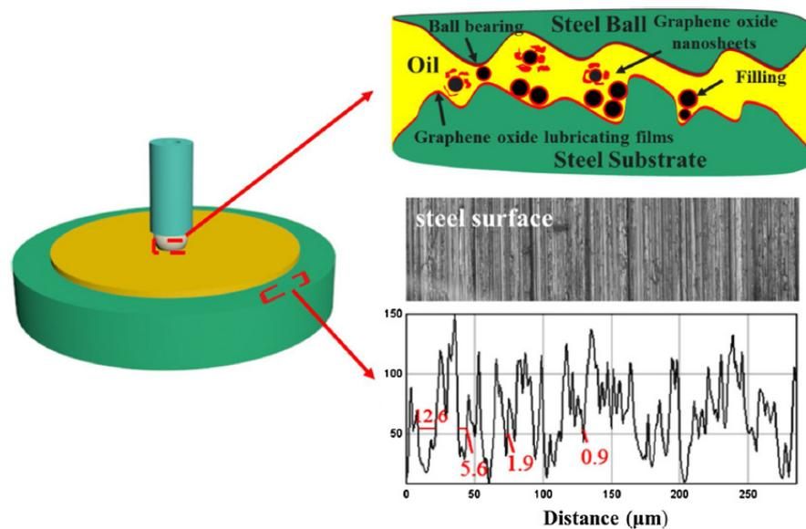
**Figure 2.** Lubrication mechanism of GO/f-CMS. Reprinted with permission from Ref. [12], Elsevier.
