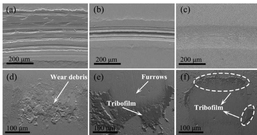
**Figure 9.** SEM images of wear tracks on: (a–c) Bottom discs; (d–f) Corresponding upper balls lubricated with different oil samples: (a,d) PAO6 oil, (b,e) PAO6 + 0.075 wt.% nano-BP, and (c,f) PAO6 + 0.075 wt.% Ag/BP. Reprinted with permission from Ref. [50], Elsevier.
