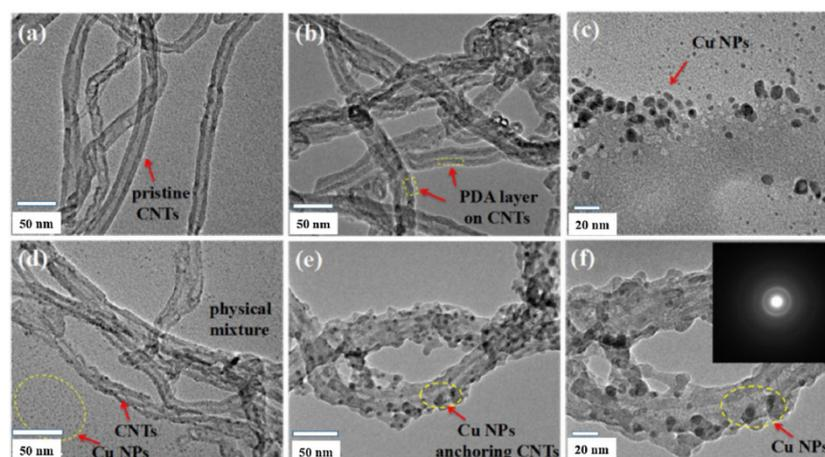
**Figure 10.** TEM images of: (a) Pure CNTs; (b) PDA/CNT composites; (c) Cu NPs; (d) Cu/CNTs; (e,f) Cu/PDA/CNT nanocomposites. Reprinted with permission from Ref. [56], Elsevier.
