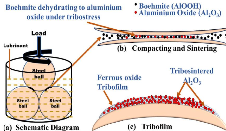
**Figure 5.** Protective film effect of  $\text{Al}_2\text{O}_3$ . Reprinted with permission from Ref. [16], Elsevier.
