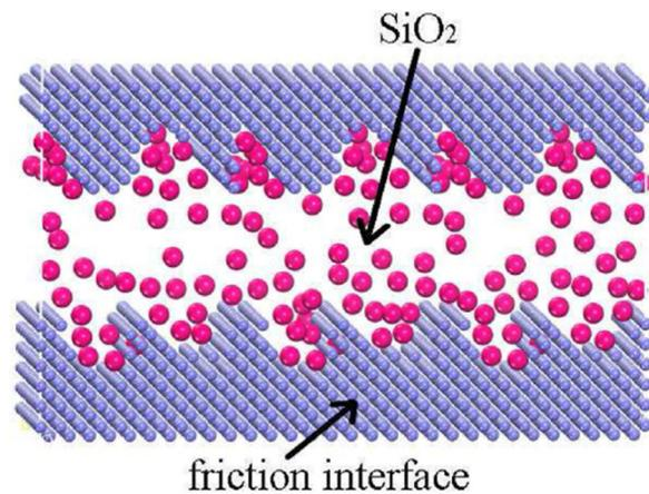
**Figure 1.** Micro-bearing effect of  $\text{SiO}_2$  nanoparticles. Reprinted with permission from Ref. [11], Elsevier.
