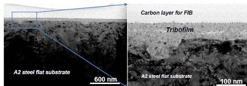
**Figure 6.** SEM images of the cross section of the tribofilm formed on a flat steel substrate lubricated by PAO+-modified silver nanoparticles. Reprinted with permission from Ref. [26], American Chemical Society.
