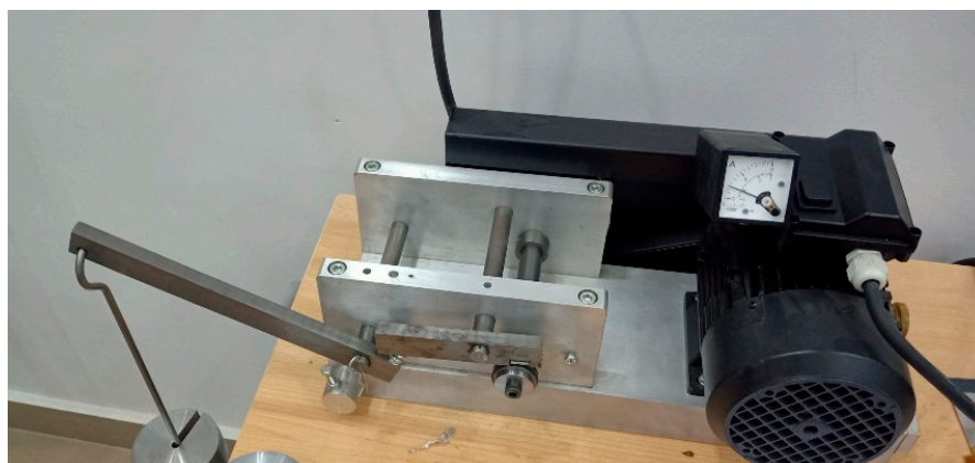
Figure 2. A customized tribotester for determining the carrying load capacity of grease samples.
