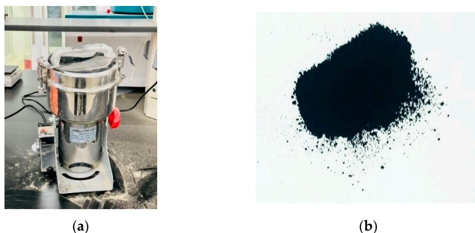
Figure 1. (a) Electric Grain Spices Multifunctional grinder (b) synthesized AC powder.
