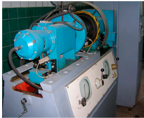
Figure 2. General view of the universal friction equipment (UMT-1) to determine the wear resistance during sliding friction.
