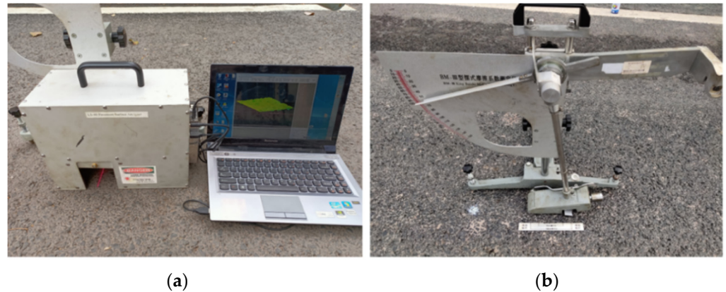
Figure 4. Field pavement data collection. (a) 3D texture data scanning; (b) road friction BPN measurement.
