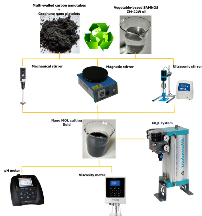
Figure 1. Vegetable-based Nano MQL cutting fluid production process.
