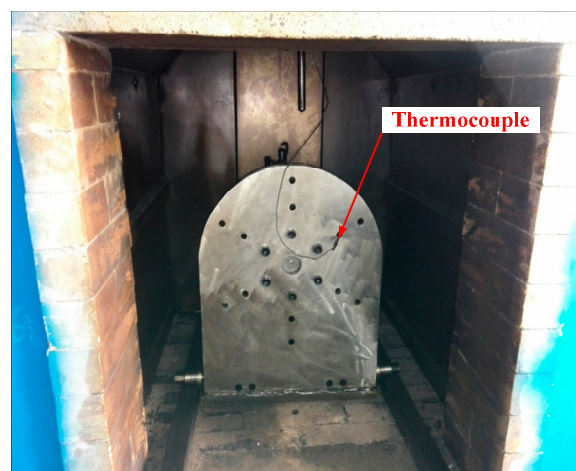
Figure 10. Fixture is laid in heating furnace.
