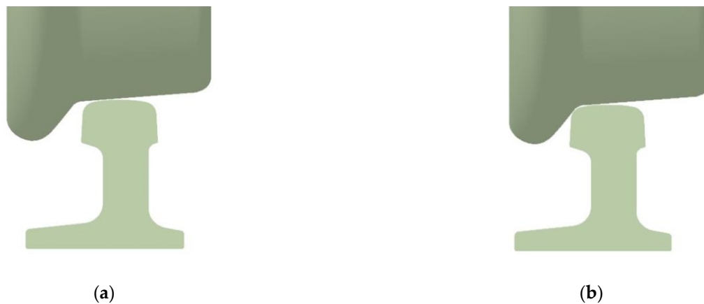
Figure 2. Wheel–rail contact status. (a) Single point of contact. (b) Two points of contact.
