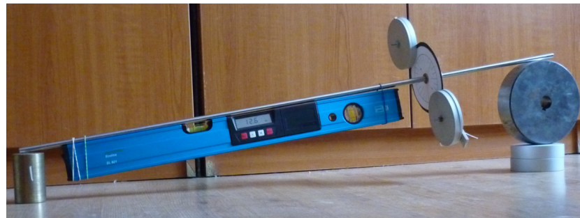
Figure 19. Finding the coefficient of friction \mu_d = \tan(\alpha) between the shaft and the bushing.
