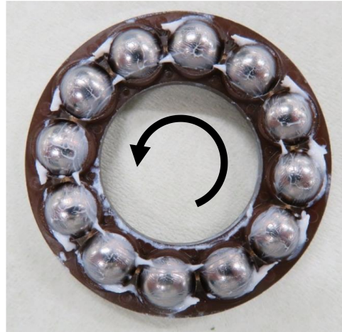
Figure 5. Photograph of grease on cage and balls after test.
