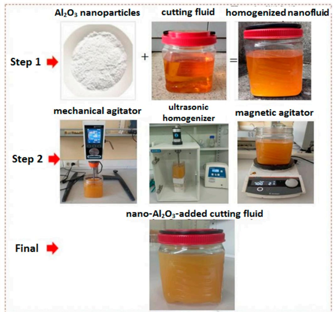
**Figure 1.** Steps applied in the preparation of vegetable-based nanofluid.
