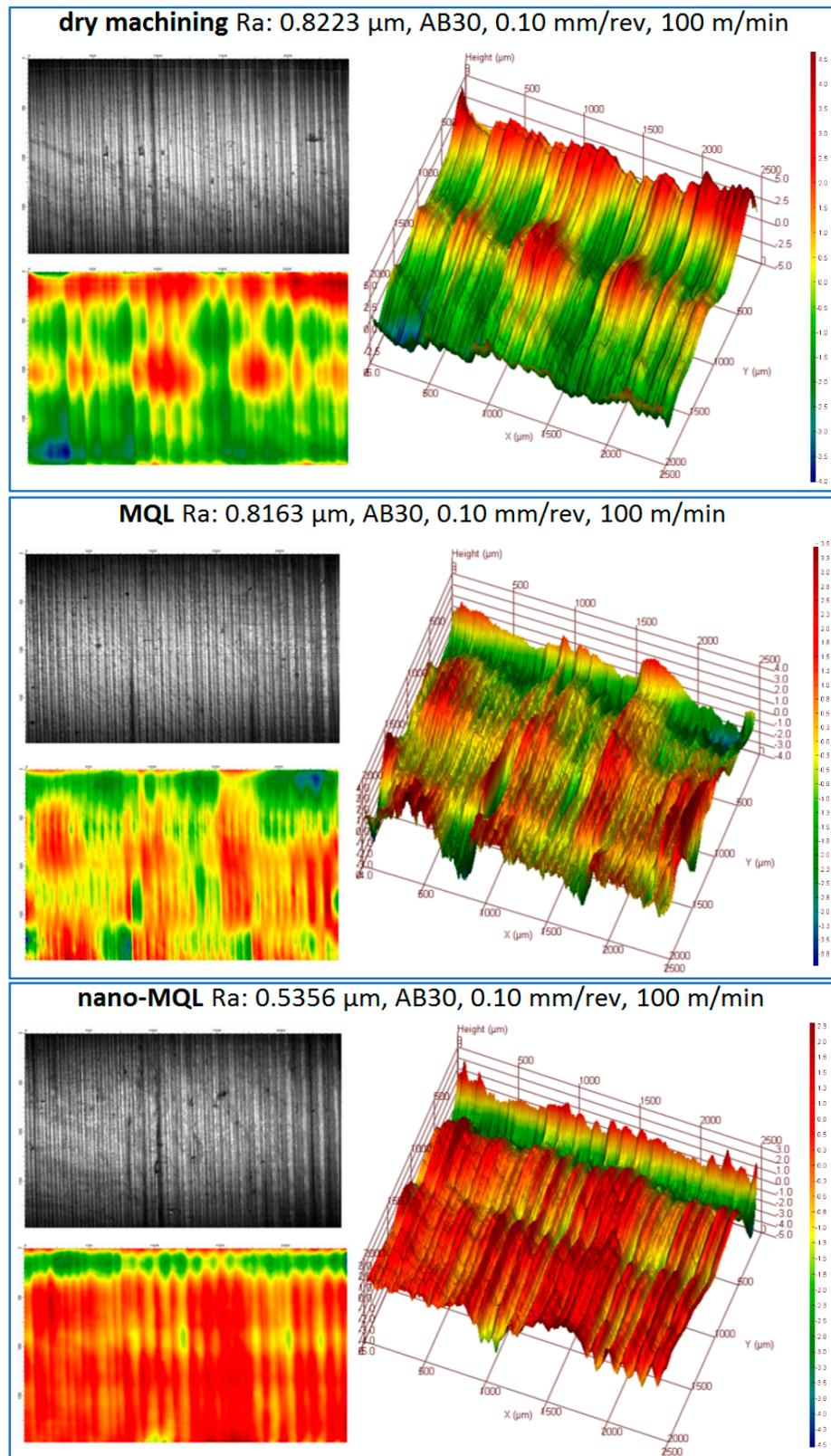
Figure 7. Pictures of machined surfaces' surface topography (AB30).
