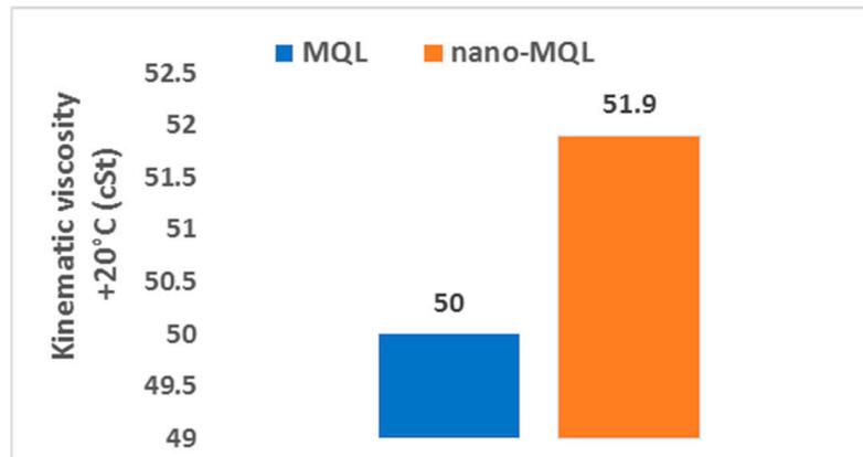
Figure 4. Kinematic viscosity values of cutting fluids used in MQL and nano-MQL methods.
