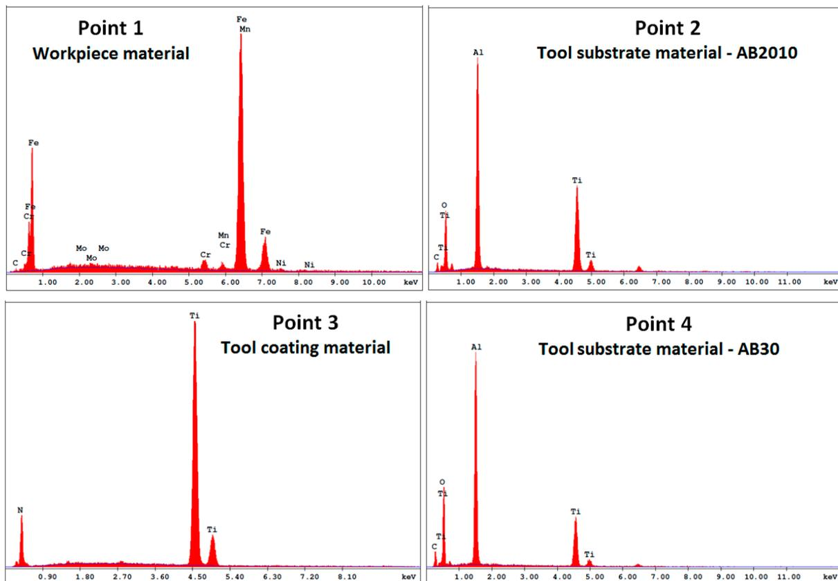
Figure 12. EDX analysis results for cutting tools.
