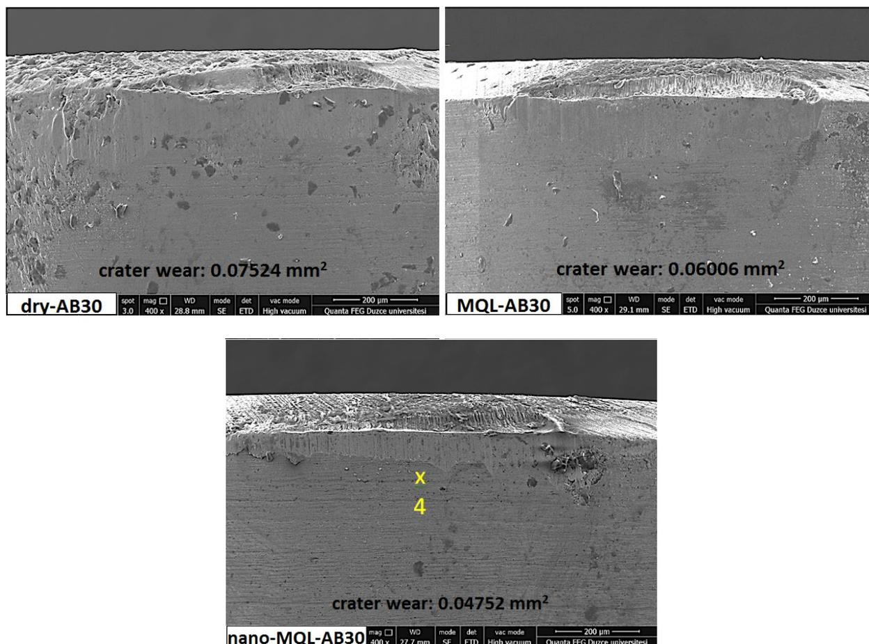
Figure 11. Crater wear changes depending on the cooling method for AB30.
