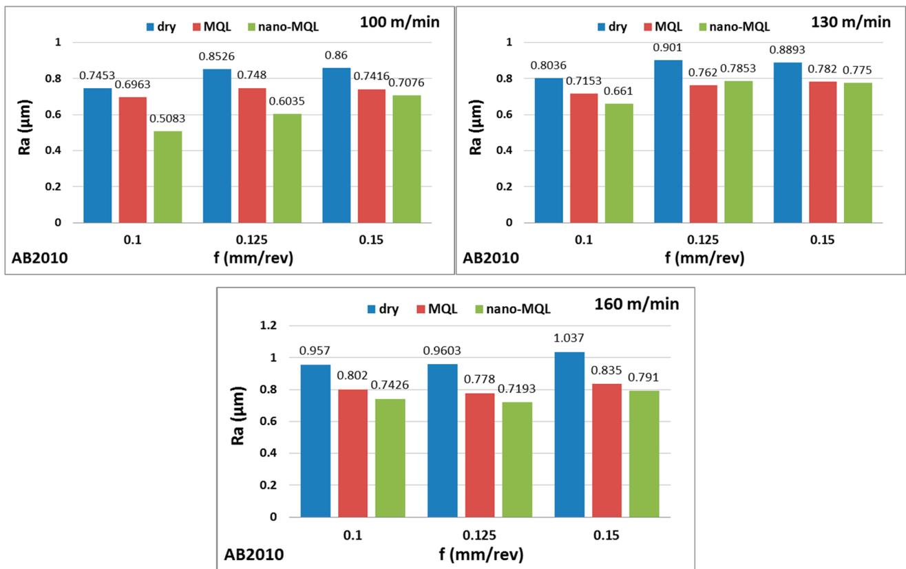
Figure 3. Ra results for AB2010 coated ceramic cutting tool.
