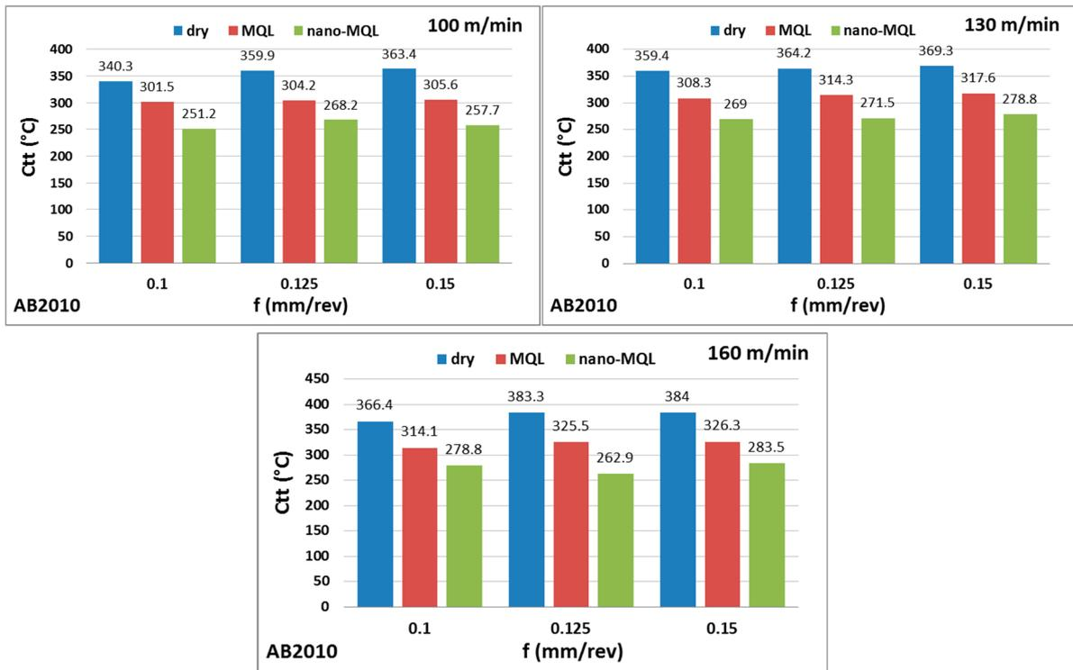
Figure 8. Cutting temperature results for AB2010 coated ceramic cutting tool.
