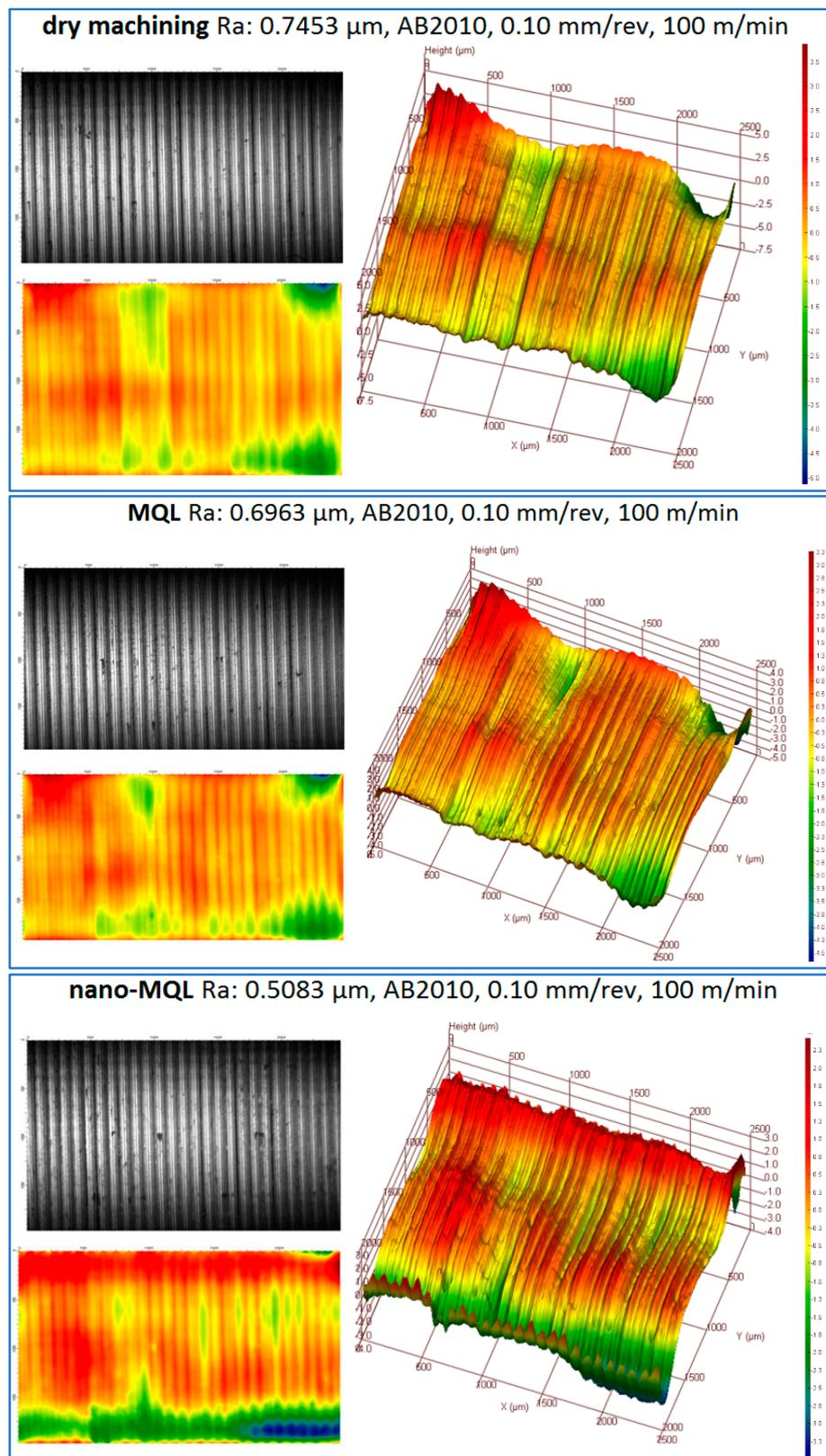
Figure 6. Pictures of machined surfaces' surface topography (AB2010).
