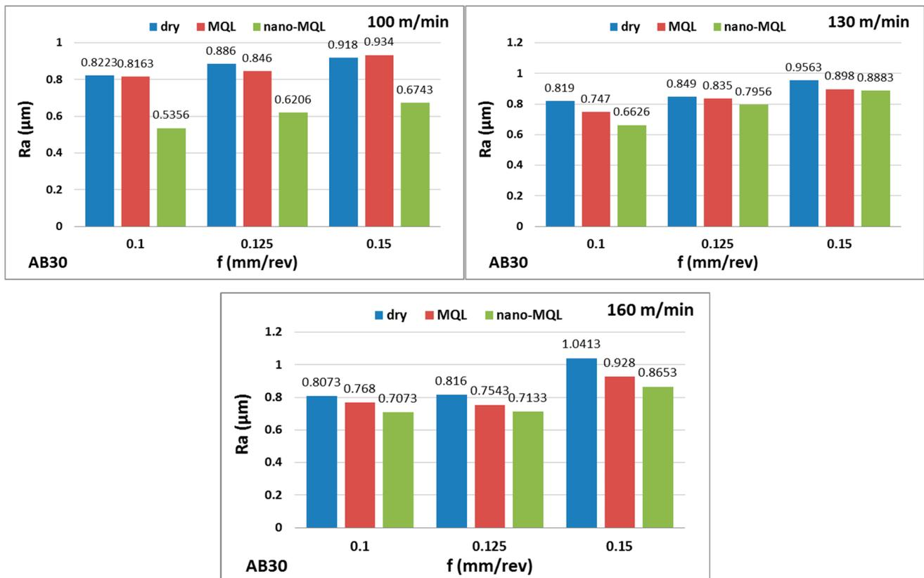
Figure 5. Ra results for AB30 uncoated ceramic cutting tool.
