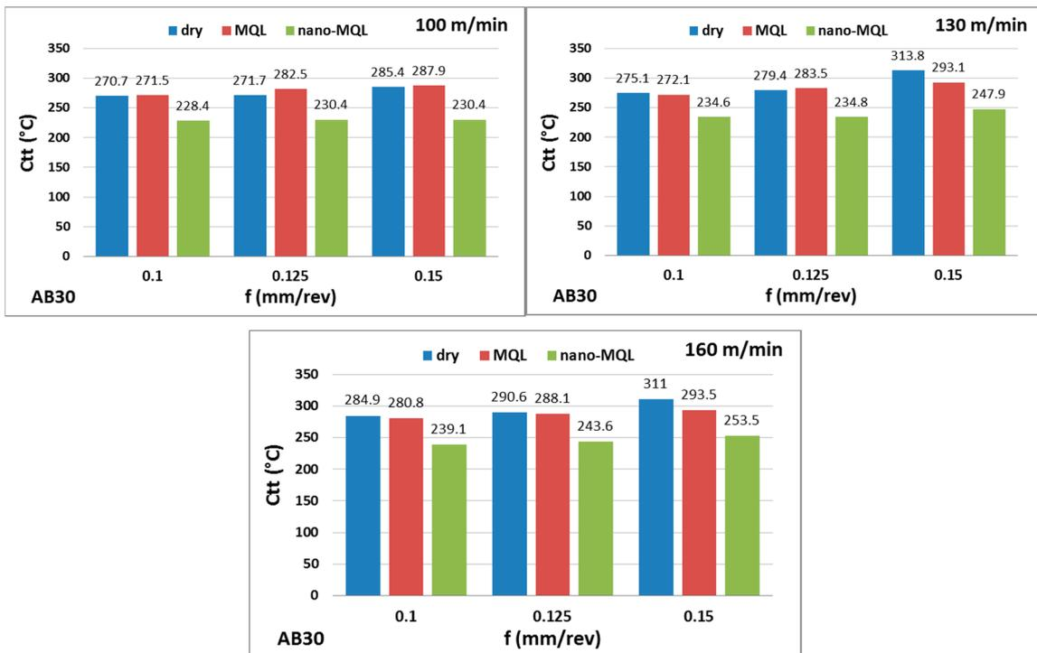
Figure 9. Cutting temperature results for AB30 uncoated ceramic cutting tool.
