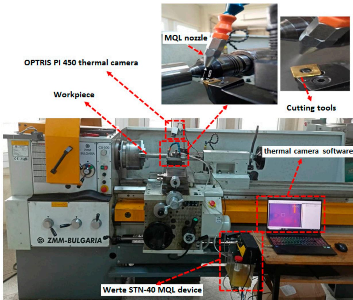
Figure 2. Experimental setup.
