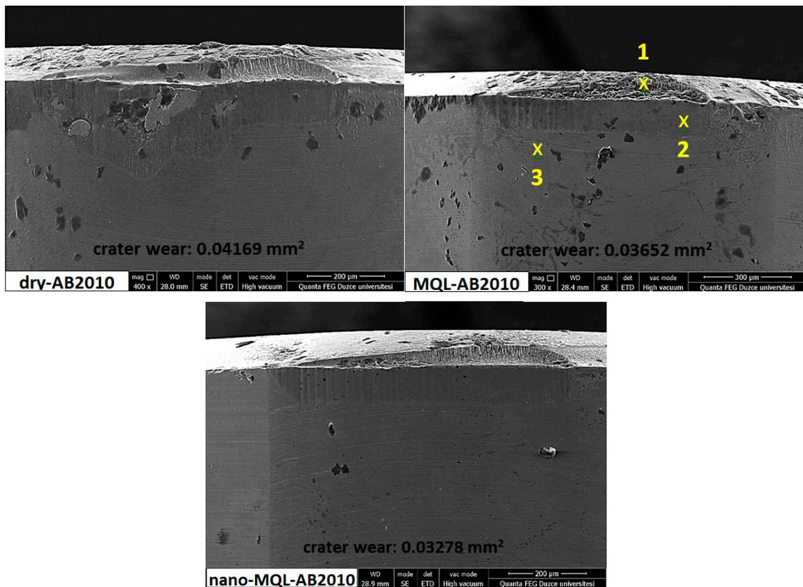
**Figure 10.** Crater wear changes depending on the cooling method used for AB2010.
