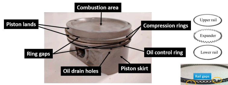
Figure 1. Sample piston (left) and three-piece oil control ring (right).
