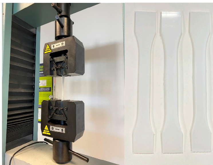
Figure 1. Tensile testing machine used and polyamide dumbbells for testing.
