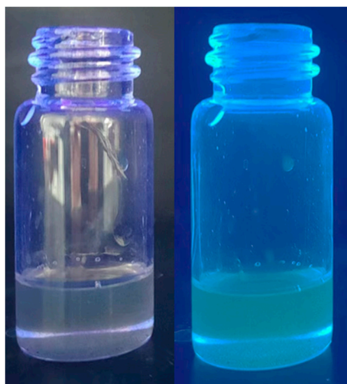
Figure 5. The prepared carbon quantum dots–liquid paraffin dispersion system.
