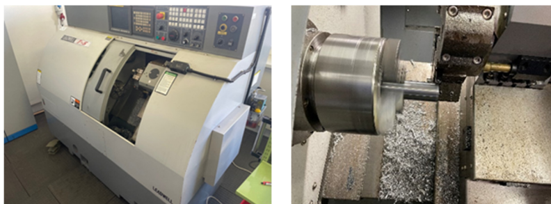
Figure 1. Technological System (TS). The TS comprises the machine (M), tool (T), workpiece (W), and fixture (F).
