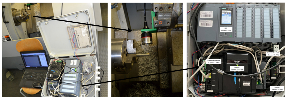
Figure 2. Mobile Measuring System (MMS).
