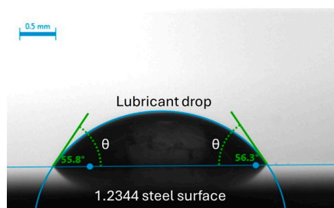
Figure 3. Contact angle \theta measurement between a polished 1.2344 steel surface and a lubricant drop.
