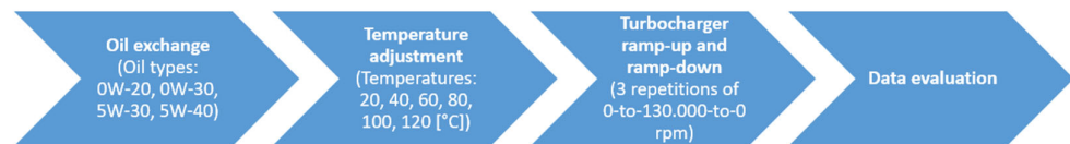
Figure 2. Flow chart of the measurement procedure.
