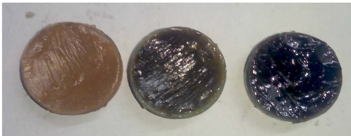
Figure 2. Fresh grease, partially grease and fully grease samples collected from wheel bearings of train.
