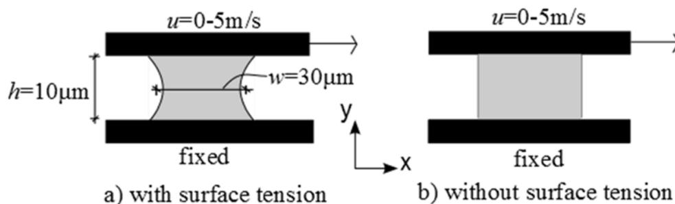
**Figure 1.** Geometry and boundary conditions for simulating a thin water film between pad and rotor.
