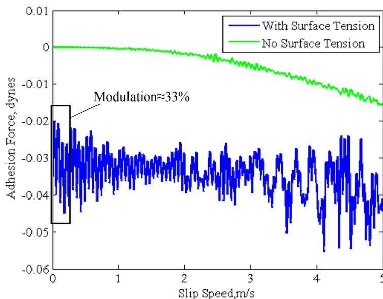
**Figure 4.** Adhesion (normal) forces vs. slip speed.
