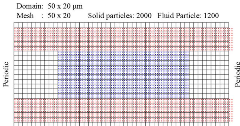
**Figure 2.** Numerical Setup in GIMP-FSI.
