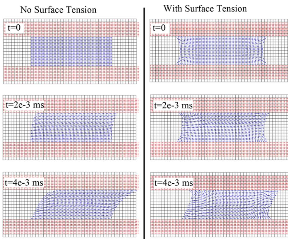
**Figure 3.** Results from GIMP-FSI for dynamic meniscus (with and without surface tension).
