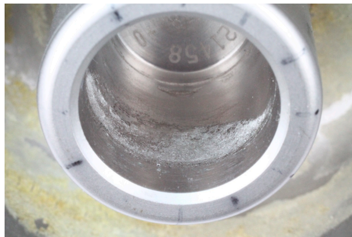
Figure 8. Crevice corrosion inside taper of large diameter femoral head.
