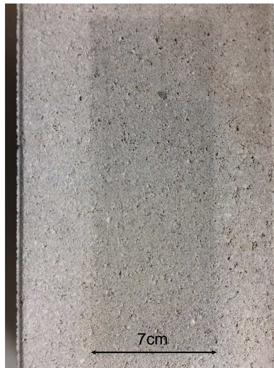
Figure 1. The concrete surface used in some of the experiments. The dark region arose from transfer of rubber material to the concrete surface during sliding at v = 1 mm/s for two cycles (each cycle is 40 cm) at T = -40 °C. Reproduced from [9], with the permission of AIP Publishing, 2018.
