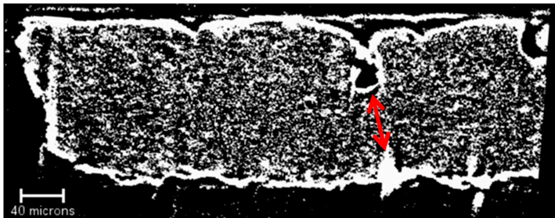
Figure 8. Images from the YZ slicing of the micro-XCT video of PLLA 24 film with 0.5 wt % INT-WS 2 (No. 7 in Table 3) with short extension before the tensile test. The white contrast is produced by the X-ray absorption of the nanotubes in the PLLA polymer.
