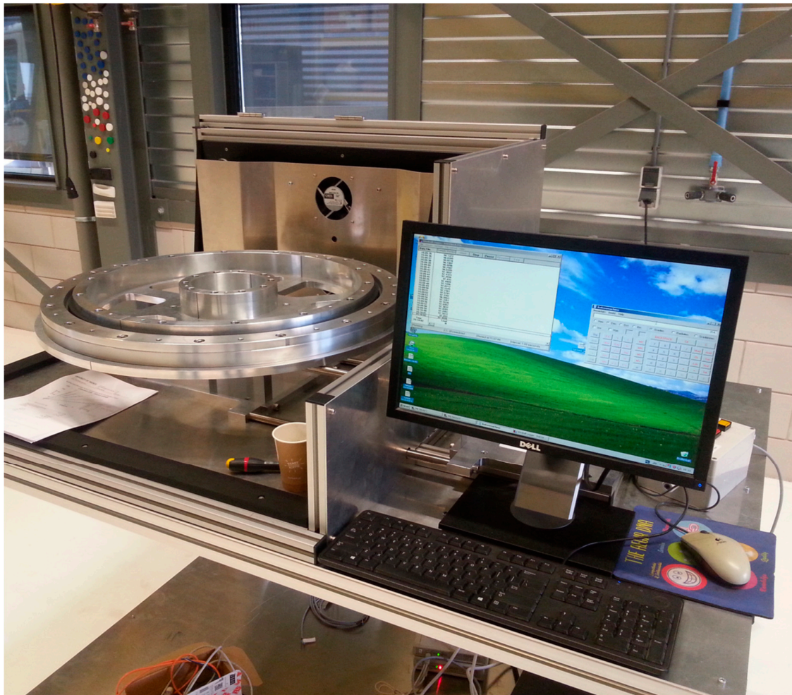
Figure 5. Split-shaft setup used for measuring the radial force exerted by the stern tube seal.
