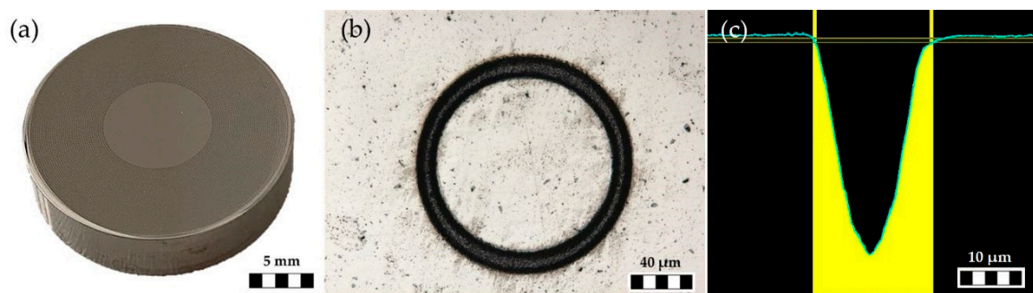
Figure 3. Microstructured CoCrMo sample. (a) Sample with global geometrical dimensions of the structured area. (b) Microscopic illustration of ring structure with diameter of 150 \mu\text{m} , gap width of 15 \mu\text{m} and depth of 10 \mu\text{m} . (c) Profilometric illustration of ring structure's well.
