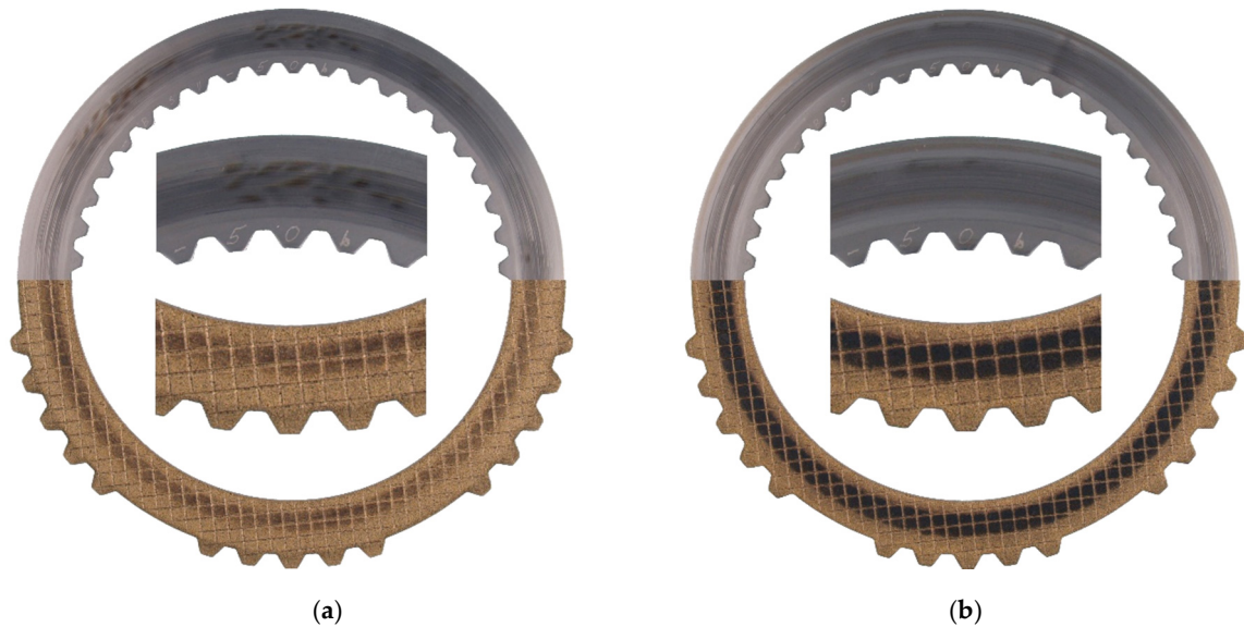
Figure 6. (a) Photos of the pre-damaged plates after load level 3; (b) photos of the pre-damaged plates after the endurance test.
