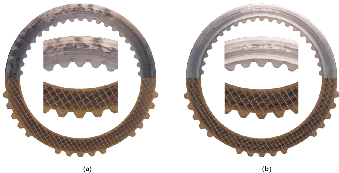
Figure 10. (a) Photo of the pre-damaged plates after load level 8; (b) photo of the pre-damaged plates after the endurance test.
