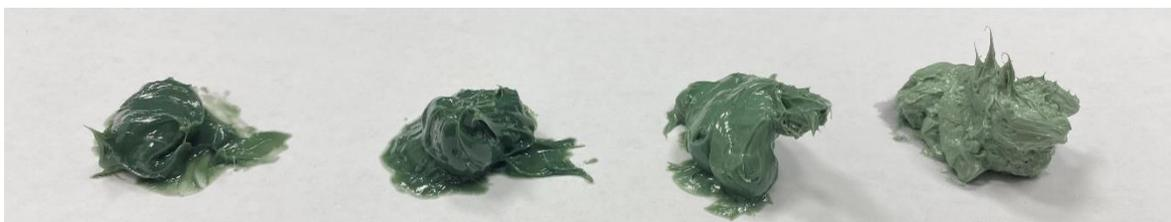
**Figure 1.** Calcium sulfonate grease contaminated with 0% (left), 1% (middle left), 10% (middle right), and 50% (right) water.
