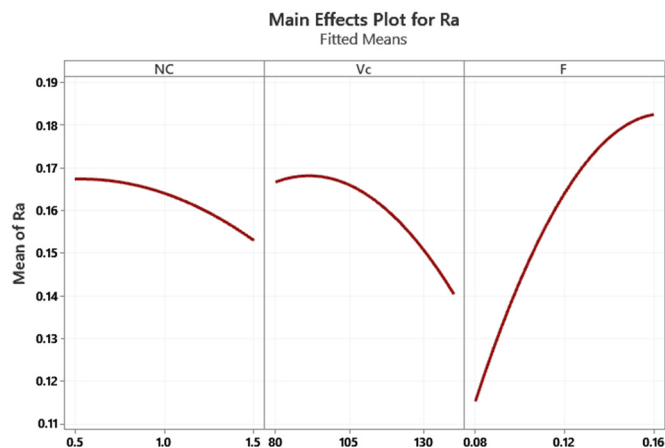
Figure 4. Main effects plot of input machining factors on surface roughness R_a .
